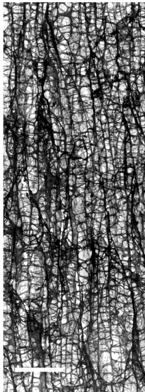
Figure 3. Quick-freeze/deep-etch TEM image of V 6 K 2 in aqueous solution at pH 4 showing the great supramolecular organization of the nanotubes, spanning several micrometers. The tubes are interconnected through three-way and multiway junctions. The apparent density of the picture belies the nature of the system because we are seeing a 2-D picture of a 3-D network. A similar effect is felt if an aerial picture is taken of a tree without leaves. The scale bar represents 500 nm.
